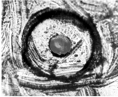
Figure 2-6. Damage from improper cleaning.
